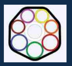
Common ducting concept: Service providers share "pathway" for building a Backbone network to save the civil works. They are assigned to use individual ducts needed and the size of the inner duct is designed for each provider's request.
